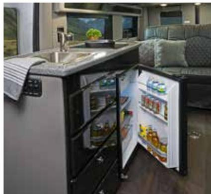
3.5 cubic foot 12v/110v refrigerator with freezer.
